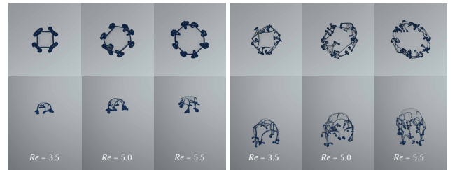
Fig. 11. Ink torus breakup at Reynolds numbers 3.5, 5.0, and 5.5. Left and right column groups show early and late frames. Top and bottom rows show top and side views. Branched blobs increase with Reynolds number.
